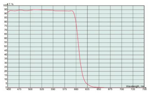
Figure 2: Typical results from coating, measured on PG&O's Perkin Elmer Lambda 950
