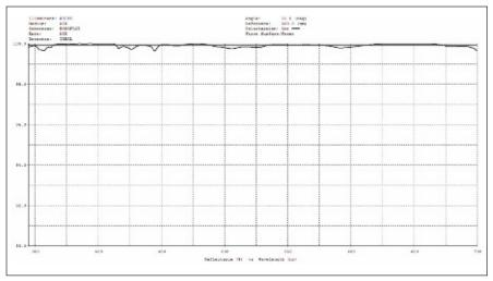
Figure 4. Optical Mirror - Reflectance vs. Wavelength Graph
