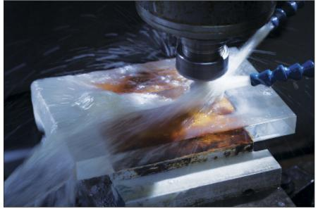
Figure 1. Machining was done on a Haas CNC machine using a custom-made fixture that held the part in place at 12.5°.
