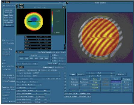
Figure 3.A 6-inch Zygo interferometer was used to verify that the surfaces met the specifications.
