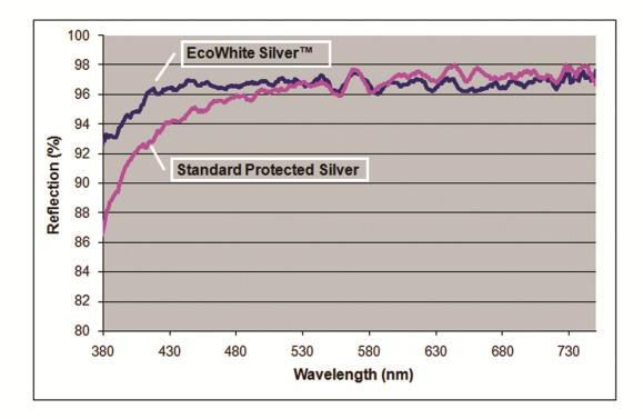
**Figure 3**: The reduction in blue roll-off using EcoWhite Silver coatings, as compared to standard protected silver coatings, saves material, reduces costs and results in better performance.
