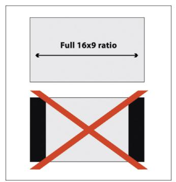
Figure 3. (Top) Illustrates full screen output with a true 16  $\times$  9 aspect ratio that is provided by the high definition (1920  $\times$  1080) camera system. (Bottom) Illustrates what can happen to the image with 3MP or higher resolution.
