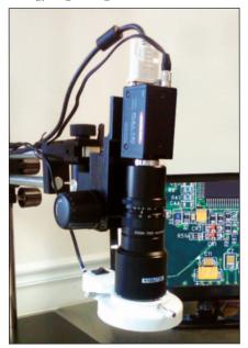
Figure 1. HD camera system designed by Dage-MTI for a circuit board inspection application.
