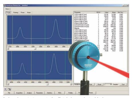
One large advantage in using a scanning slit profiler is that beams can be viewed directly with little or no power attenuation needed. Courtesy of Ophir-Spiricon.
