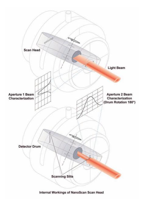
The scanning slit beam profiler moves a narrow slit in front of a photodetector through the beam under analysis. Courtesy of Ophir-Spiricon.
