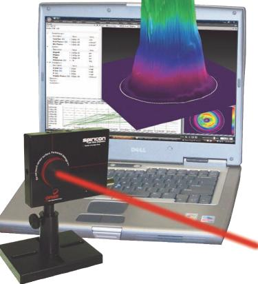
Camera-based systems capture the entire beam profile by using a CCD or CMOS camera, which provides a real-time 2- and 3-D image of the beam. Images courtesy of Ophir-Spiricon.
