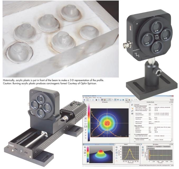
For Thorlabs' beam profilers, optional extension kits for automated M<sup>2</sup> beam quality analysis are available. The software package can be downloaded for free from the company's website. Shown here is the BC100 series camera profiler. Images courtesy of Thorlabs.
