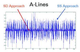
Figures 3a and 3b: Figure 3a (top) illustrates the difference between the wide fluctuations of phase stability in a commercial swept source OCT system compared to that of a Spectral-Domain system (photodiode array with fixed grating spectrometer). Figure 3b (bottom) illustrates the phase difference between consecutive A-lines recorded by the same two systems.
