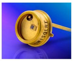
half intensity beam angle of 110 degrees and is conveniently packaged in a 2-lead TO-39 can with an isolated case. Forward voltage is 1.75 volts (typical) to 2 volts (maximum); reverse breakdown voltage ranges from a minimum of 5 volts to 30 volts (typical). The rise and fall times for the high-temperature wide angle IRLED is 20 nanoseconds, respectively.
