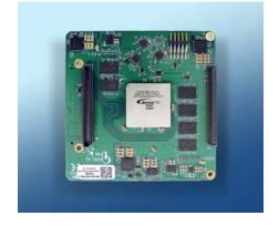
The A10 board supports both OpenCL<sup>™</sup> and high-level synthesis (HLS) tools for accelerating design cycles and targeting C/C++ code to the FPGA. Critical Link's innovative MitySOM-A10S-DSC processor with embedded Linux provides operating system support, versatility, and ease of customization for complex imaging platforms.
