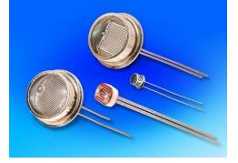
CdS photoresistors are ideal for street and solar lighting, audio compression and flame detection,
