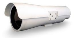
The 640 x 512 pixel resolution, indium antimonide (InSb) detector with a 15-micron pitch is optimized to operate in the MWIR spectrum (3 - 5  $\mu$ m), commonly considered the best waveband for imaging in marine and high-humidity environments. Other all-weather applications for the 550CZ-18 camera system include border protection, vessel traffic monitoring, critical infrastructure protection, and airport perimeter surveillance.
