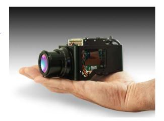
Designed to optimize the detection and visualization of hydrocarbon gas leaks, such as methane, propane, butane, and many more, the "hot-MWIR" Ventus OGI is a lightweight, low-power camera core that can be integrated onto fixed-mounted, continuous-monitoring systems or used in gimbals or in enclosures for unmanned aerial system platforms.
