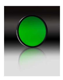
These ultra-steep filters with >OD6 blocking out of the band and state-of-the-art center wavelength tolerances of  $< \pm 0.3\%$  offer the highest transmission levels available with a passband average of >95% (see graphic). The new filters aid in the fluorescent detection of the virus and cover most common fluorophores for single and multiplexed qPCR filters, including FAM, Cy5, HEX, JOE, ROX, TexasRed®, and TRITC.
