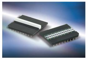
For X-ray or gamma-ray applications, there are three scintillator-mounting options: bismuth germinate (BGO), cadmium tungstate (CdWO<sub>4</sub>) and caesium or cesium iodide (CsI). When coupled with a scintillator, the OSI's silicon detector arrays map any medium- or high-radiation energy over to the visible spectrum via scattering effect. For larger-scale assembly, multiple arrays may be installed to achieve optimum results.
