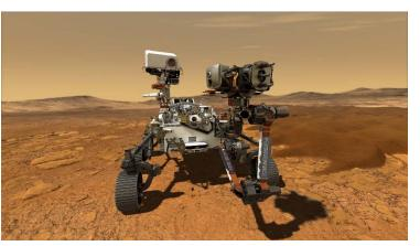
Alluxa's filters help enable non-contact detection and characterization of organics and minerals on Mar's surface. Developed in conjunction with NASA's Jet Propulsion Lab (<u>https://www.jpl.nasa.gov</u>) in Pasadena, California, the SHERLOC instrument, part of the Perseverance payload, is a Deep UV (DUV) resonance Raman and fluorescence spectrometer that will scan for past life on Mars and help identify rock samples for possible return to Earth.
