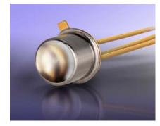
Electro-optical characteristics (at 25° C) include emission wavelengths ranging from 260 nm (minimum) to 270 nm (maximum), with a typical peak emission at 265 nm. The spectral bandwidth is 13 nm (typical), the half-intensity beam angle is only 9 degrees, forward voltage is 5 volts (typical) to 6.5 volts (maximum), and capacitance is 350 pF (typical). The new, narrow-spectral-output UVLED offers long-lifetime operation and is well-suited for disinfection applications.
