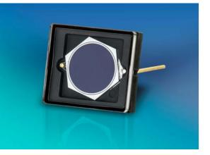
The circular active area device is specially designed for high-energy detection, such as laser power monitoring applications. Under test conditions at 254 nm, the UVG20S detector's responsivity ranges from 0.105 A/W (minimum) to 0.115 A/W (typical). Shunt resistance is 100 MOhms (typical) and reverse breakdown voltage is 50 volts (typical). At 0 V bias, capacitance is 1.5 nF (typical) and response time is 4 microseconds (typical).
