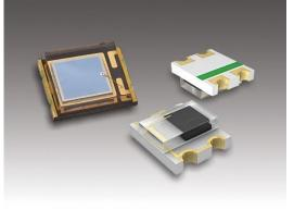
Advanced Photonix's silicon and InGaAs SMT detectors are offered in various wavelengths ranging from Ultraviolet (UV) to Near Infrared (300 nm to 1700 nm). The photodetectors range in varying active area sizes from 0.185 mm<sup>2</sup> up to 8.07 mm<sup>2</sup> to meet customers' specific needs. The company's SMT optical sensors also feature small footprints, low dark current and capacitance, and high sensitivity.
