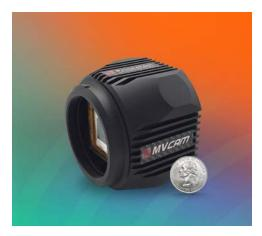
(fps), with higher frame rates for user-selectable regions of interest (ROI). At 12  $\mu$ m pixel pitch, the MVCam InGaAs image sensor yields extremely low dark current and high quantum efficiency, providing sensitivity across the SWIR and visible wavelength bands from 0.4 to 1.7  $\mu$ m. The standard camera configuration uses a single-stage thermoelectric cooler (with no moving parts), integrated in a sealed package to stabilize the image sensor at 20°C.
