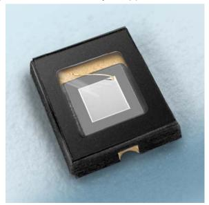
The NXIR-RF100C has an active area of 1 mm $^2$  in a small 3 mm x 3.5 mm surface-mount package. The new device has high responsivity of 0.62 A/W @ 850 nm and 0.35 A/W @ 1064 nm. It also has low capacitance of 3 pico-farads (pF) at 0 volts, high shunt resistance, greater than 200 M $\Omega$ , and very low dark current at 0.1nA. Opto Diode's NXIR-RF100C detectors are available in high volume on tape and reel.
